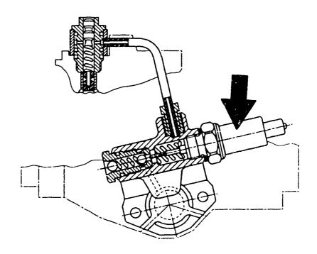
Position speed-control lever against rated-speed adjusting screw. At the given speeds, the supply pump pressure profile and the timing-device profile must be attained within the adjustment tolerance (setting not in brackets).
